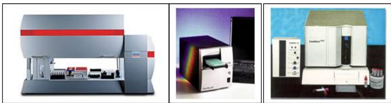
Figure 5: AFRRRI’s high-throughput microsphere immunoassay analysis system. The photographic images show the analytical system that robotically processes blood samples to measure protein biomarker changes predictive of radiation exposure using the microsphere immunoassay. See manuscript text for details. Components of this system were derived from a previous published study [Blakely 2003b].
